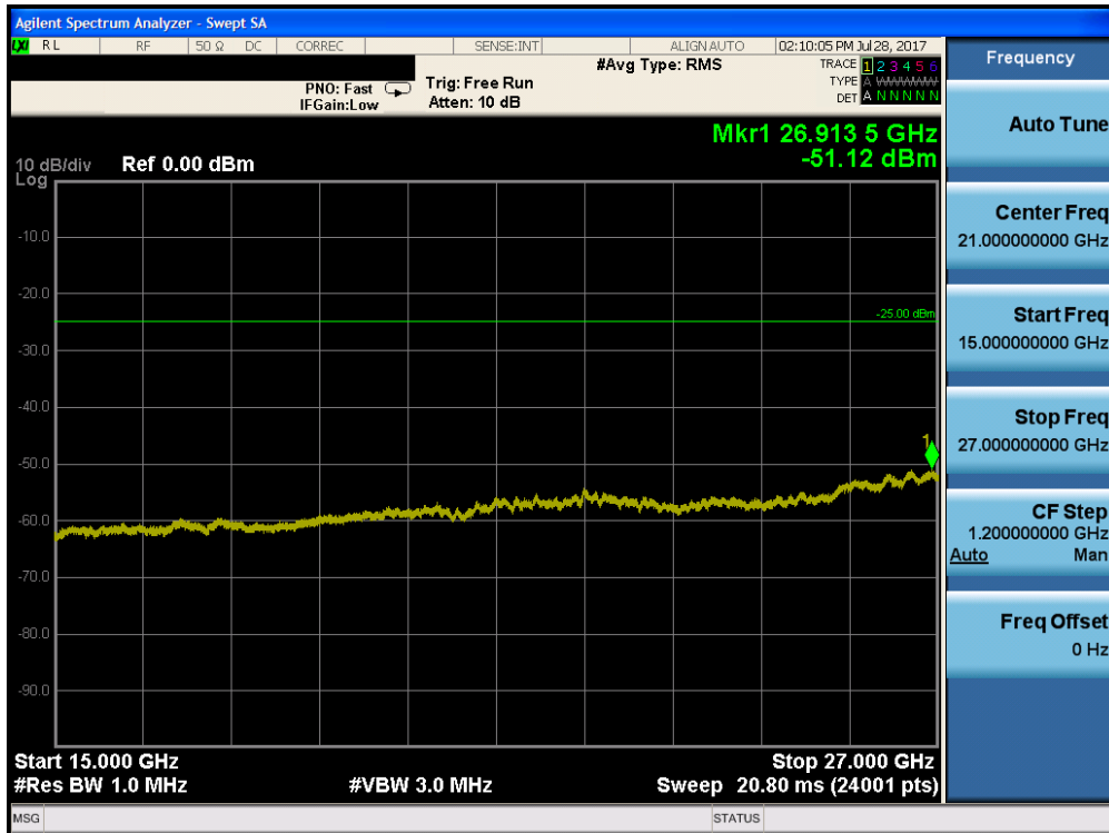
Plot 7-34. Conducted Spurious Plot (Band 7 – 5.0MHz QPSK – RB Size 1, RB Offset 0 – High Channel)
