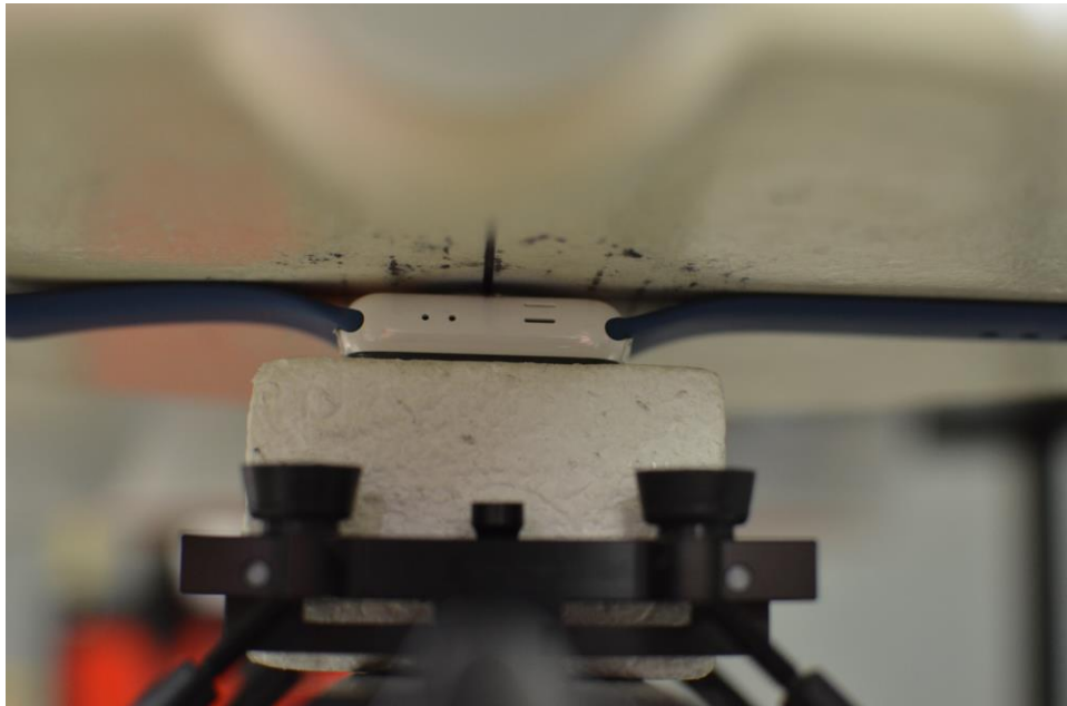
SAR Test Setup Photo 18: Ceramic with Sport wristband, Back side at 0.0 cm
