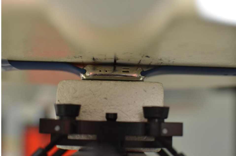
SAR Test Setup Photo 15: Stainless Steel with Sport wristband, Back side at 0.0 cm
