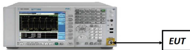
Figure 7-4. Test Instrument & Measurement Setup
