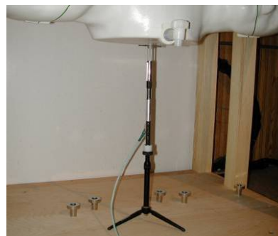
Figure 9-2 System Verification Setup Photo
