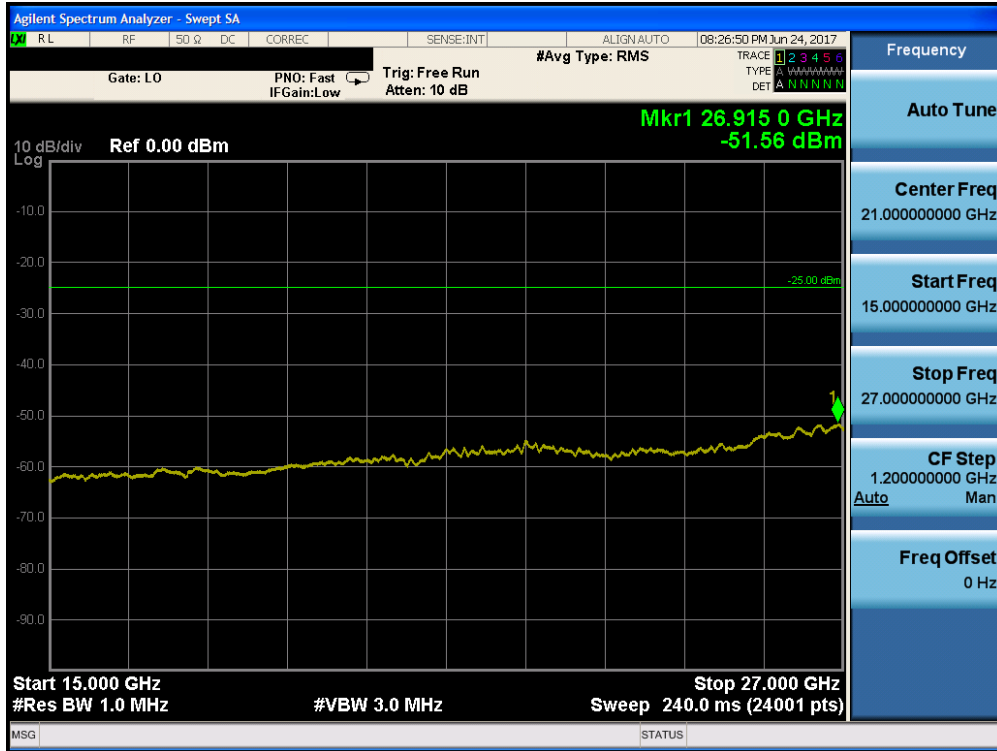
Plot 7-17. Conducted Spurious Plot (Band 41 – 10.0MHz QPSK – RB Size 1, RB Offset 0 – High Channel)
