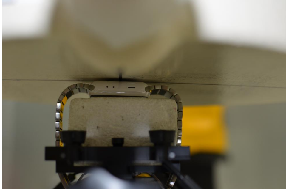
SAR Test Setup Photo 17: Ceramic with Metal Links wrist band, Back side at 0.0 cm
