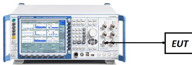
Figure 7-4. ERP/EIRP Measurement Setup
