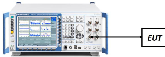
Figure 7-4. ERP Measurement Setup
