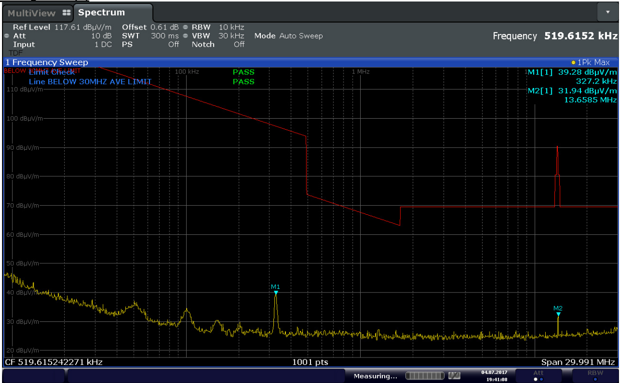
Plot 7-1. Radiated Spurious Plot 9kHz – 30MHz (CE A 848kbps, Pol. X)
