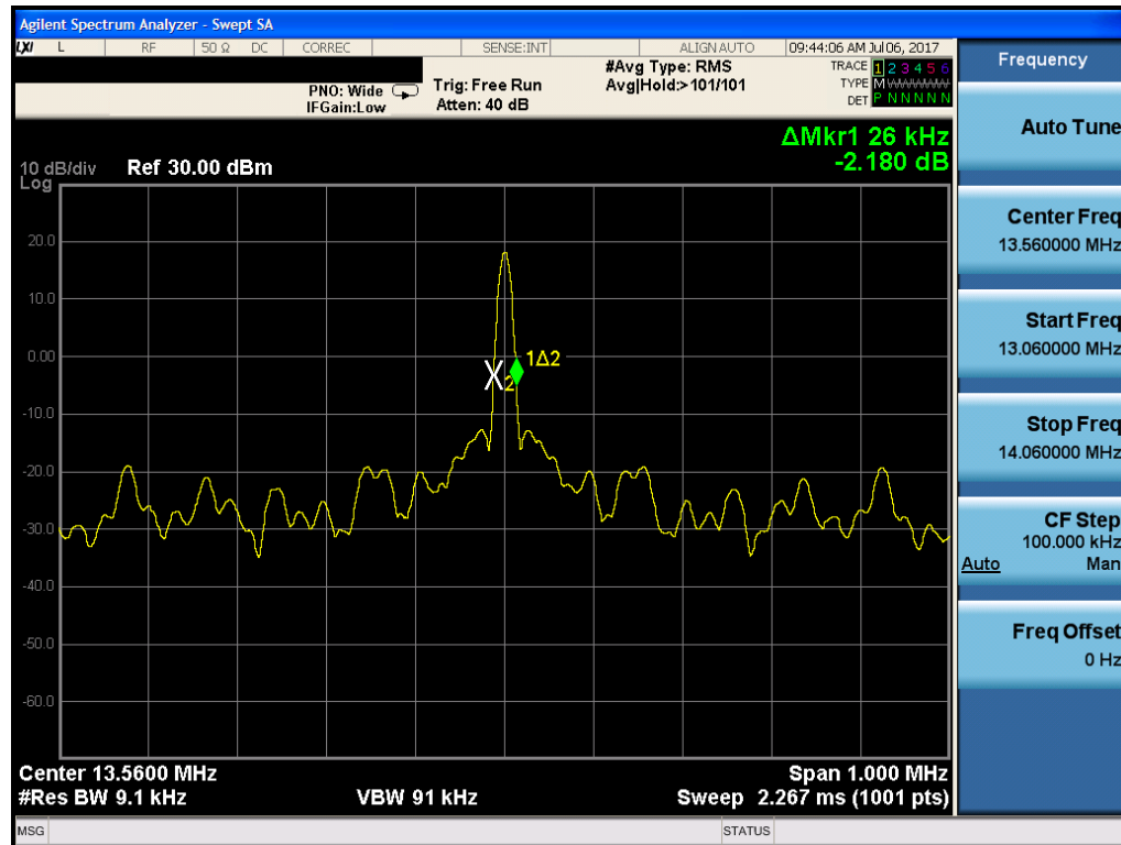
Figure 7-3. 20dB Bandwidth Plot (CE B 848kbps)
