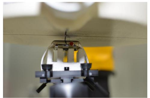
SAR Test Setup Photo 6: Stainless Steel with Sport wristband, Front side at 1.0 cm
