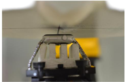
SAR Test Setup Photo 2: Aluminum with Metal Links wristband, Front side at 1.0 cm
