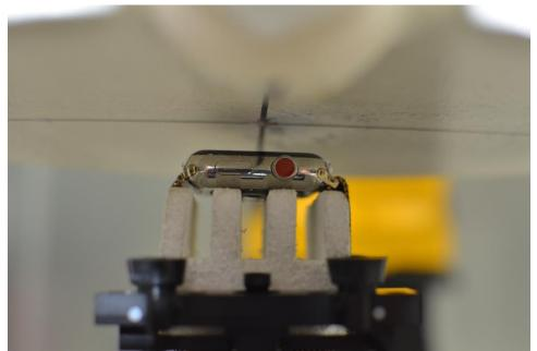
SAR Test Setup Photo 4: Stainless Steel with Metal Loop wristband, Front side at 1.0 cm
