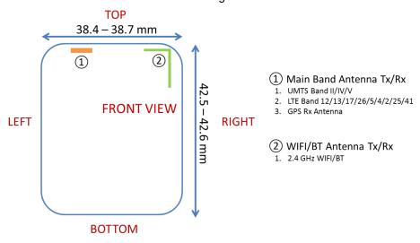
Figure F-1 DUT Antenna Locations
