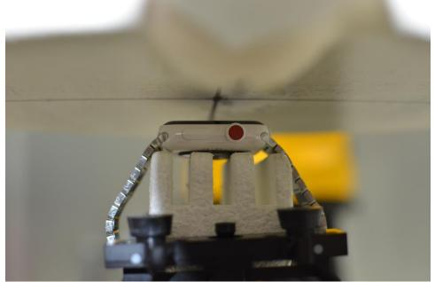
SAR Test Setup Photo 8: Ceramic with Metal Links wristband, Front side at 1.0 cm
