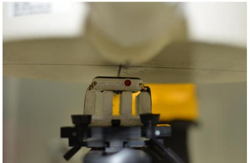
SAR Test Setup Photo 7: Ceramic with Metal Loop wristband, Front side at 1.0 cm
