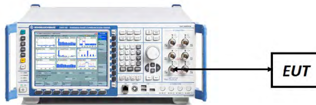
Figure 7-5. ERP/EIRP Measurement Setup
