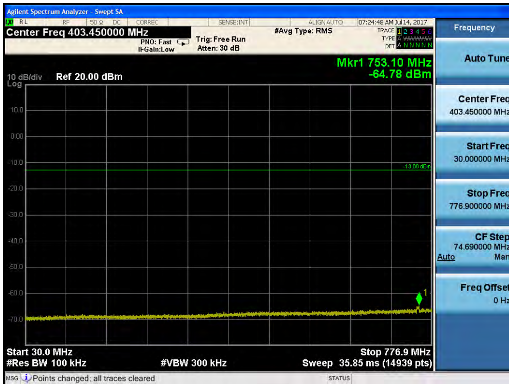
Plot 7-62. Conducted Spurious Plot (Band 13 – 5.0MHz QPSK – RB Size 1, RB Offset 0 – Low Channel)
