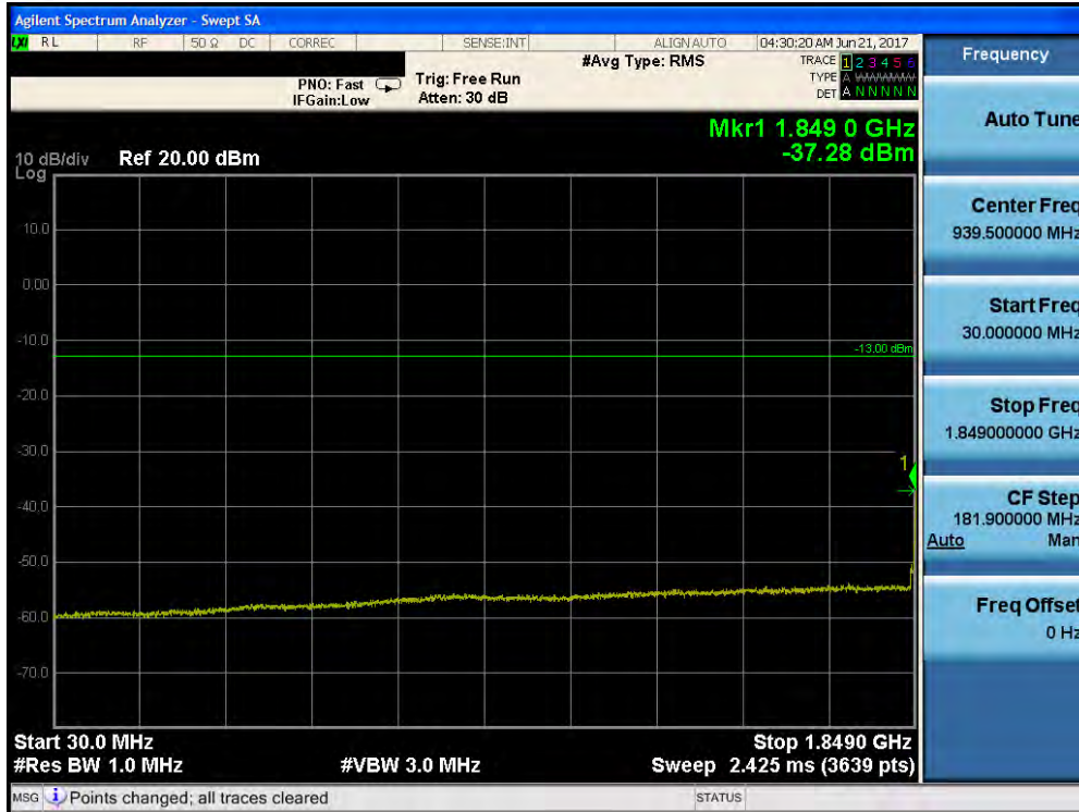
Plot 7-89. Conducted Spurious Plot (Band 2/25 – 1.4MHz QPSK – RB Size 1, RB Offset 0 – Low Channel)
