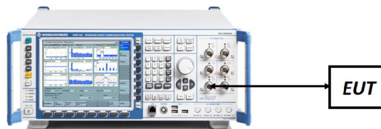
Figure 7-5. ERP/EIRP Measurement Setup
