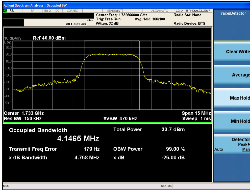
Plot 7-2. Occupied Bandwidth Plot (AWS WCDMA Mode – Ch. 1413)
