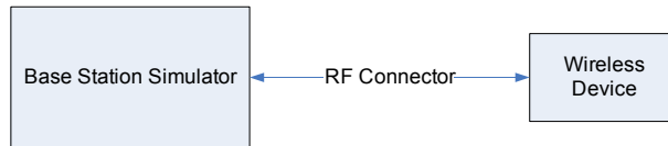
Figure 8-1 Power Measurement Setup
