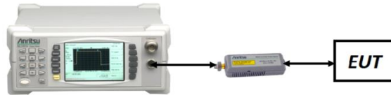
Figure 7-3. Test Instrument & Measurement Setup (Average Power Measurement)
