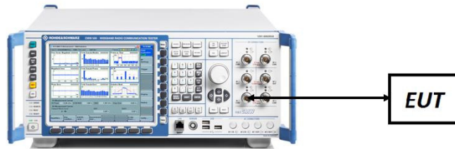
Figure 7-4. Conducted Power Measurement Setup
