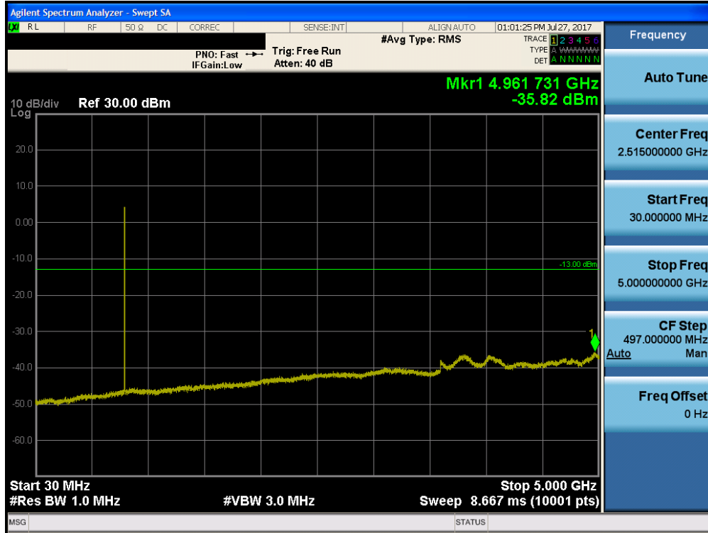
Plot 7-9. Conducted Spurious Plot (5MHz QPSK – RB Size 1, RB Offset 0 – Low Channel)
