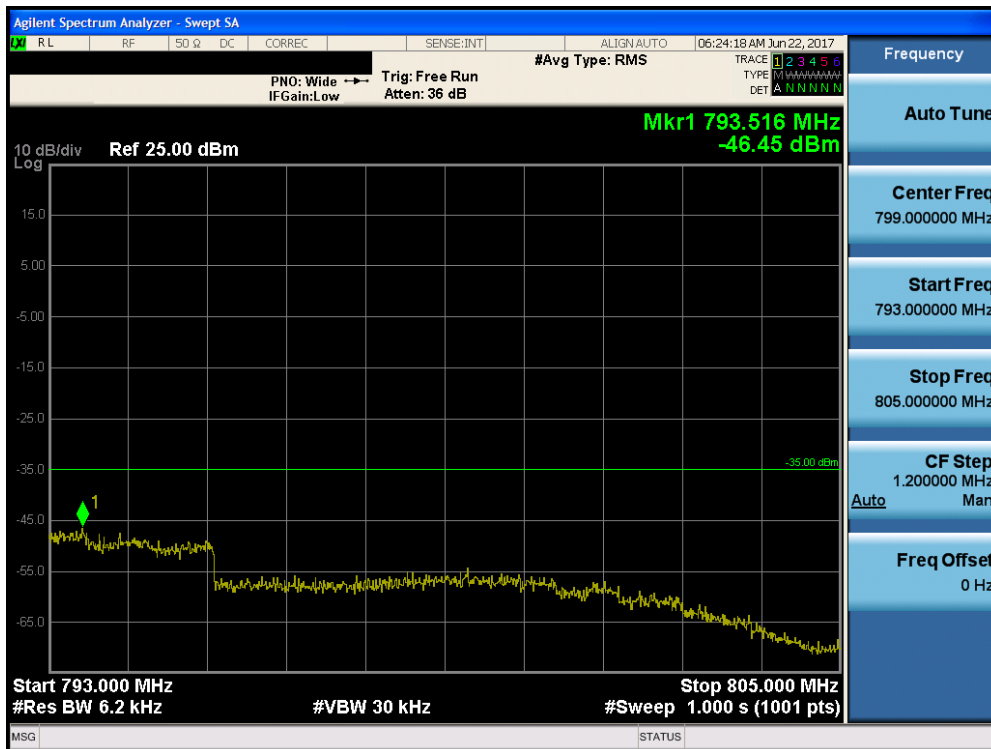
Plot 7-124. Upper Emission Mask Edge Plot (Band 13 – 10.0MHz QPSK – RB Size 50)
