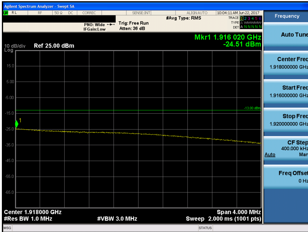
Plot 7-186. Upper Extended Band Edge Plot (Band 25 – 15.0MHz QPSK – RB Size 75)
