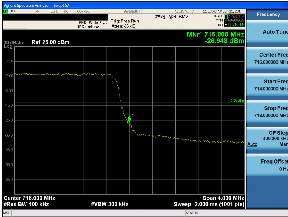
Plot 7-113. Upper Band Edge Plot (Band 12/17 – 5.0MHz QPSK – RB Size 25)
