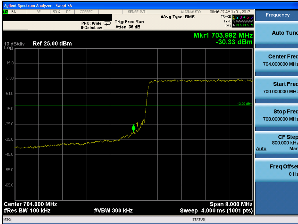
Plot 7-115. Lower Band Edge Plot (Band 17 – 10.0MHz QPSK – RB Size 50)
