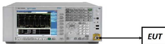
Figure 7-4. Test Instrument & Measurement Setup
