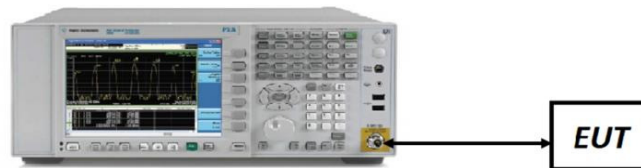
Figure 7-1. Test Instrument & Measurement Setup
