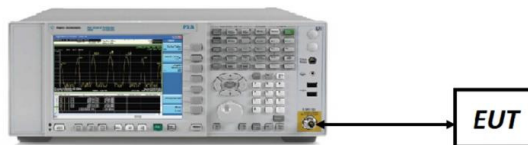
Figure 7-5. Test Instrument & Measurement Setup
