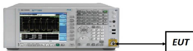
Figure 7-1. Test Instrument & Measurement Setup
