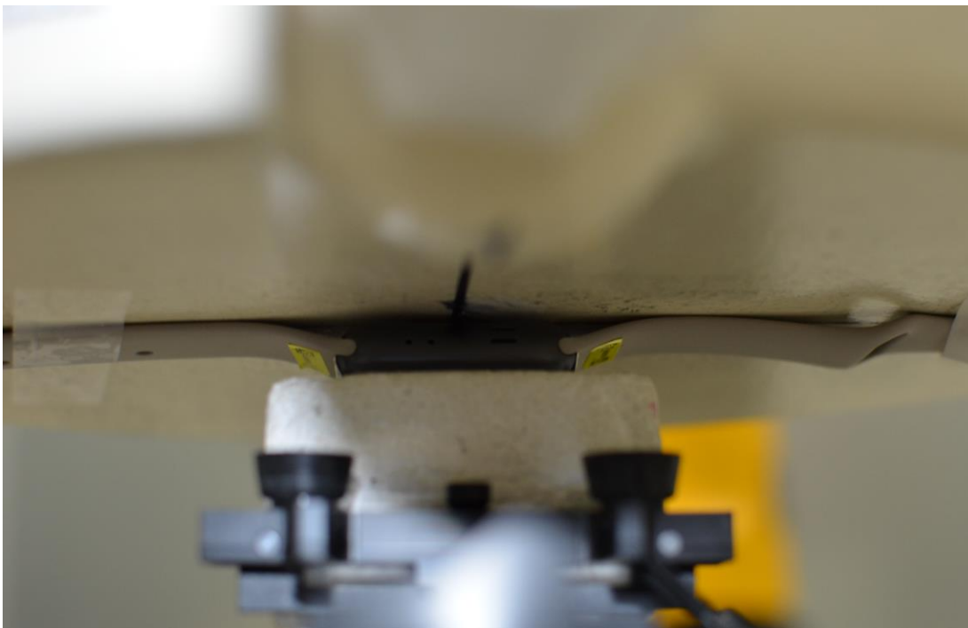
SAR Test Setup Photo 6: Aluminum back side at 0.0 cm with sport wrist band
