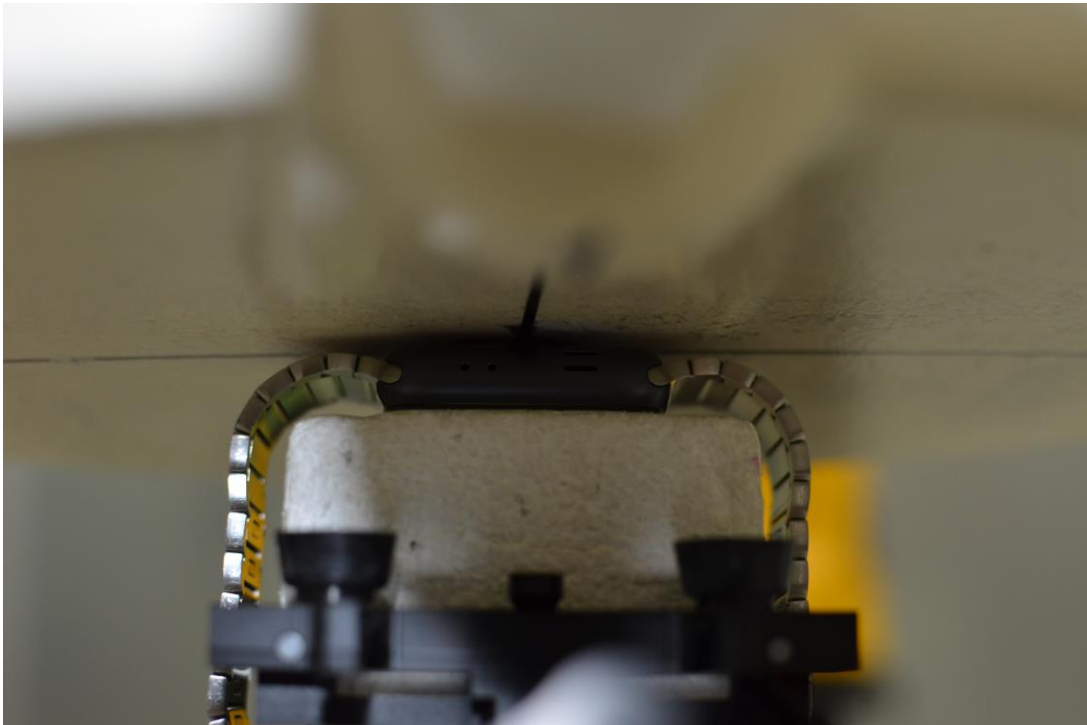
SAR Test Setup Photo 5: Aluminum back side at 0.0 cm with metal links wrist band
