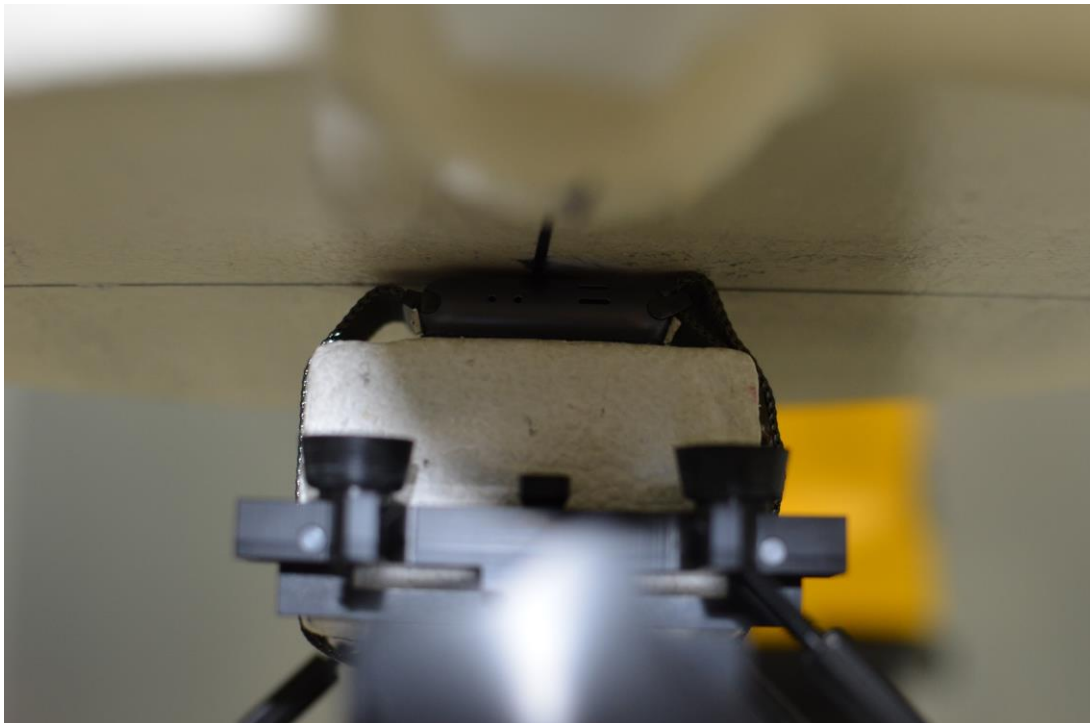
SAR Test Setup Photo 4: Aluminum back side at 0.0 cm with metal loop wrist band
