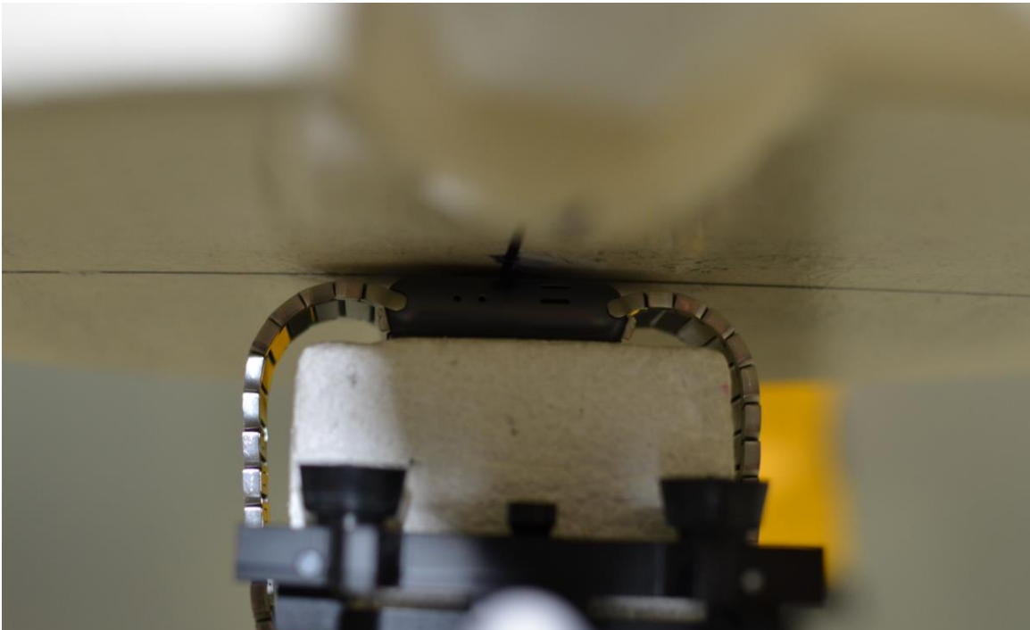
SAR Test Setup Photo 5: Aluminum back side at 0.0 cm with metal links wrist band
