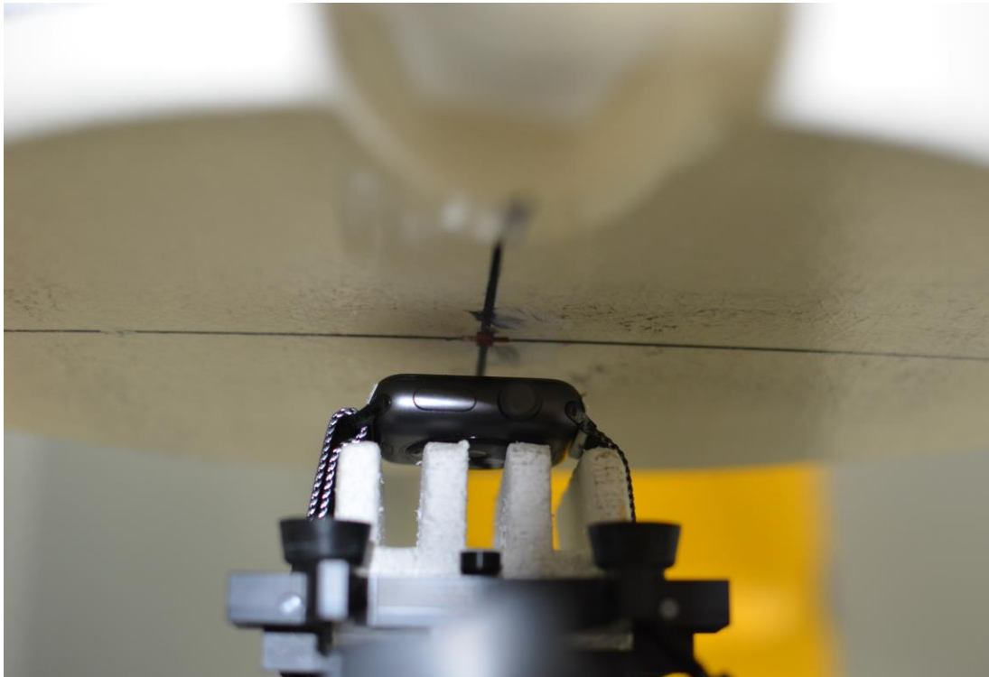
SAR Test Setup Photo 1: Aluminum front side at 1.0 cm with metal loop wrist band
