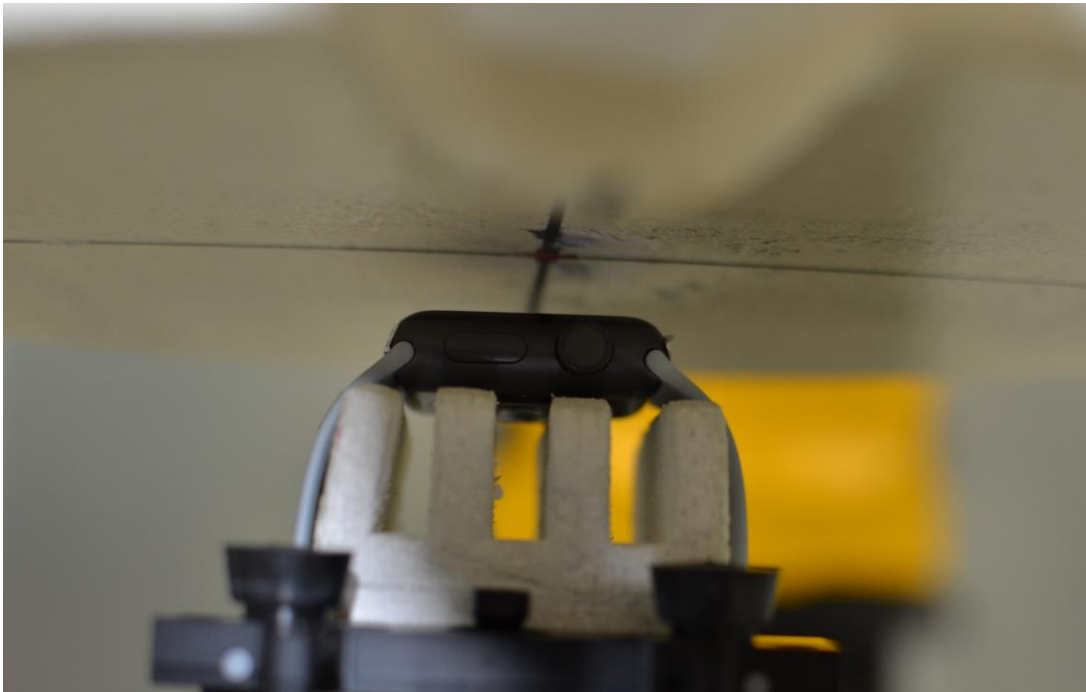
SAR Test Setup Photo 3: Aluminum front side at 1.0 cm with sport wrist band
