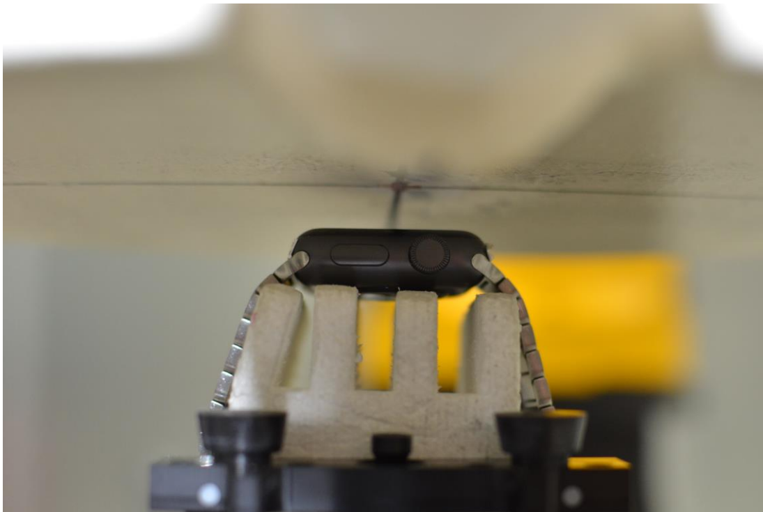
SAR Test Setup Photo 2: Aluminum front side at 1.0 cm with metal links wrist band
