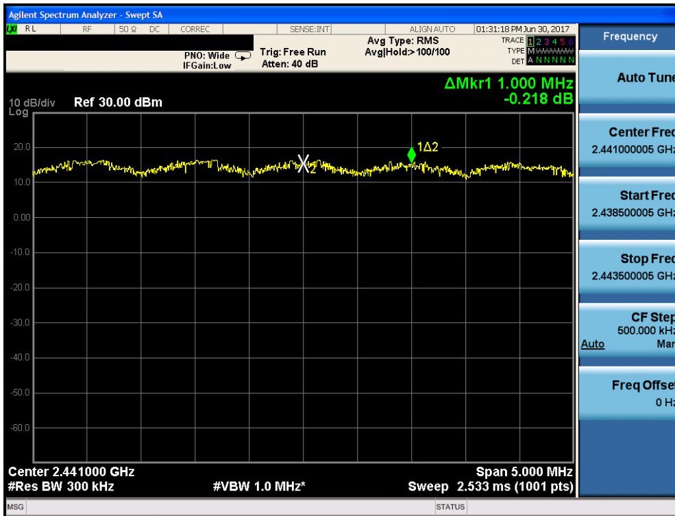
Plot 7-42. Channel Spacing Plot (Bluetooth, 8DPSK, ePA)
