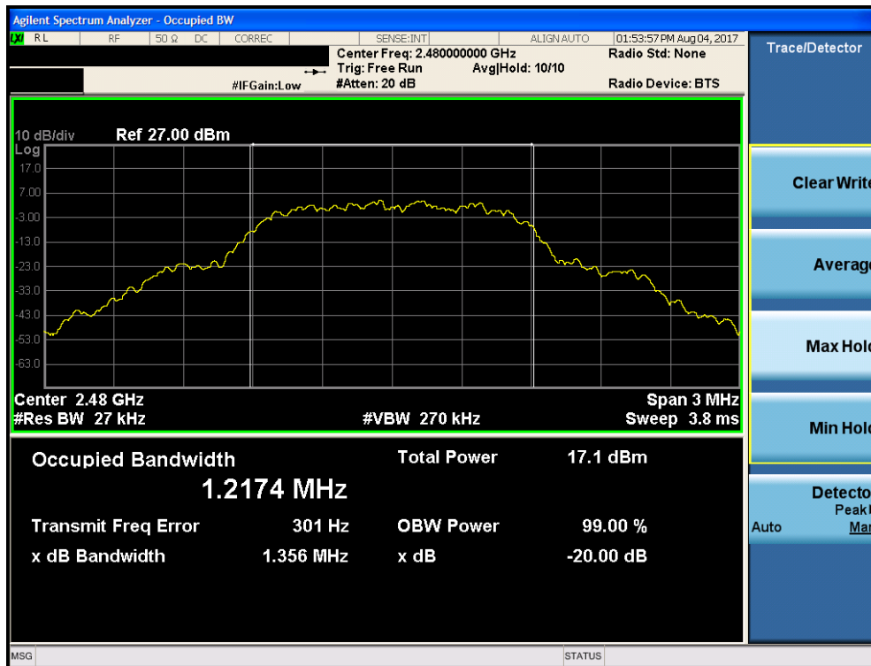
Plot 7-12. 20dB Bandwidth Plot (Bluetooth, 8DPSK, iPA – Ch. 78)
