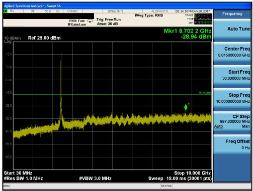
Plot 7-33. Conducted Spurious Plot (802.11b - Ch. 6)
