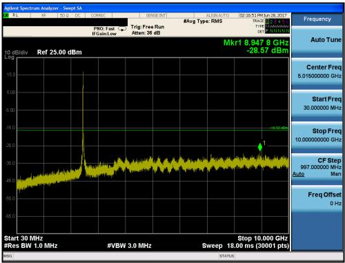
Plot 7-35. Conducted Spurious Plot (802.11b - Ch. 11)
