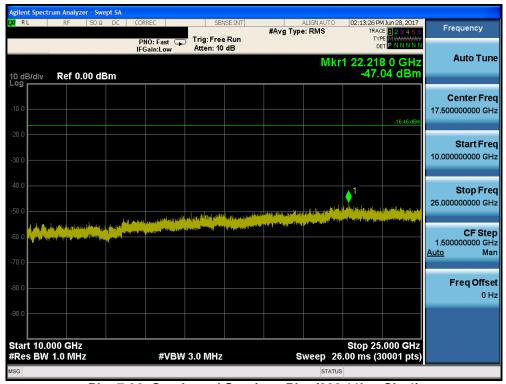
Plot 7-32. Conducted Spurious Plot (802.11b - Ch. 1)
