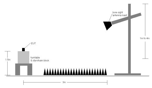
Figure 7-6. Test Instrument & Measurement Setup
