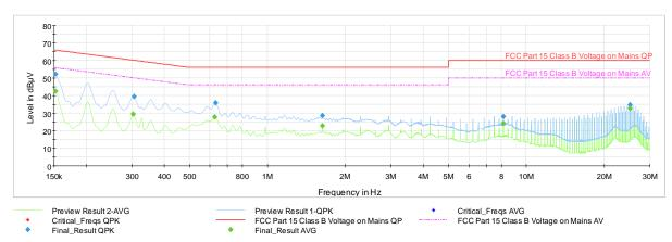
Plot 7-50. Line Conducted Plot with 802.11b (L1)
