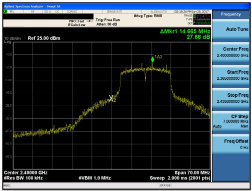
Plot 7-27. Band Edge Plot (802.11n (2.4GHz) - Ch. 1)
