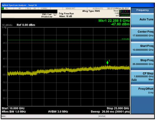
Plot 7-36. Conducted Spurious Plot (802.11b - Ch. 11)
