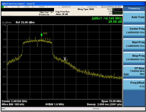
Plot 7-29. Band Edge Plot (802.11n (2.4GHz) - Ch. 12)
