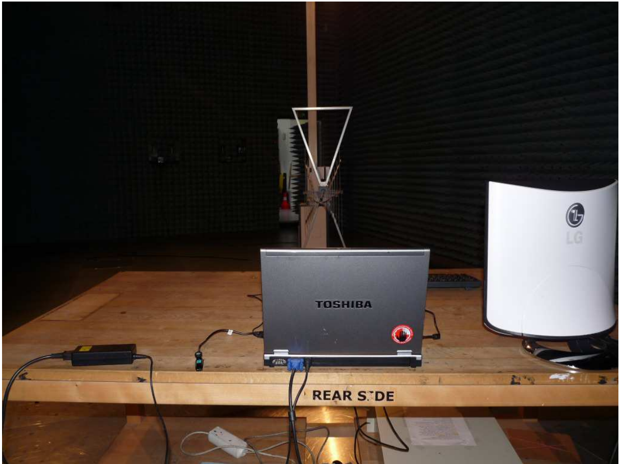
setup for the test radiated emissions. EUT powered by USB
