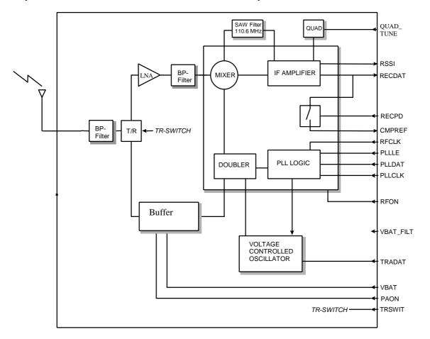
This document describes the functionality of the RF part of Activa. The RF is based on the LMX 3162 single chip RF from National Semiconductor. Two to other main components are the ALPS UREA630 VCO.
