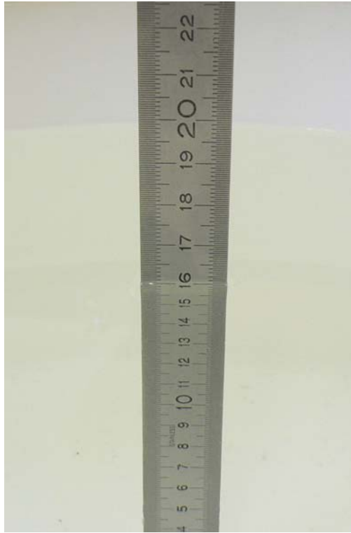
Fig. 15: Liquid depth for 2450 MHz, flat part of the SAM phantom using head simulating liquid.
