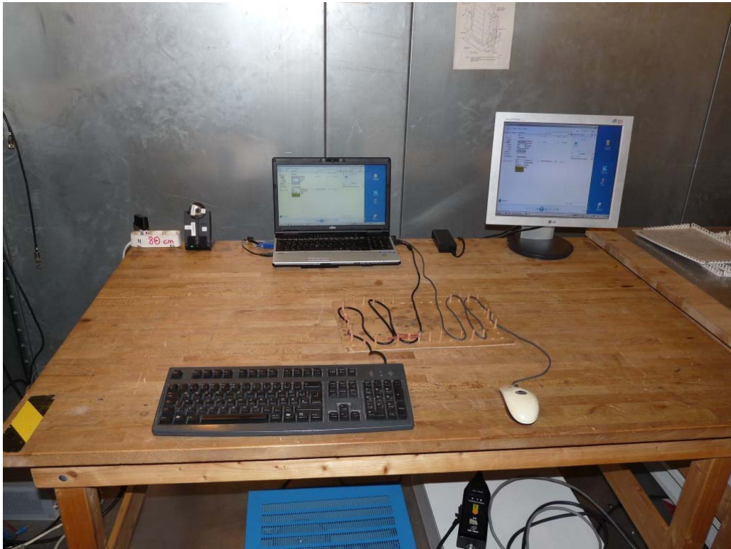
Photo 2: Test setup for conducted measurements (computer peripheral setup, EUT supplied by AC/DC adapter. USB-cable from computer as data traffic my streaming music, unintentional radiator §15)
