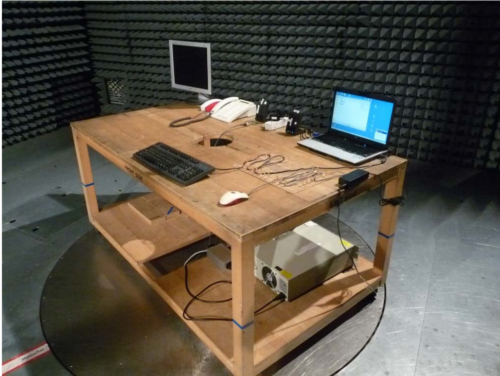
Photo 3: Test setup for radiated measurements (AC Port (power line and computer peripheral setup), EUT supplied by AC/DC adapter. Data traffic on USB-Cable by streaming music, unintentional radiator §15)
