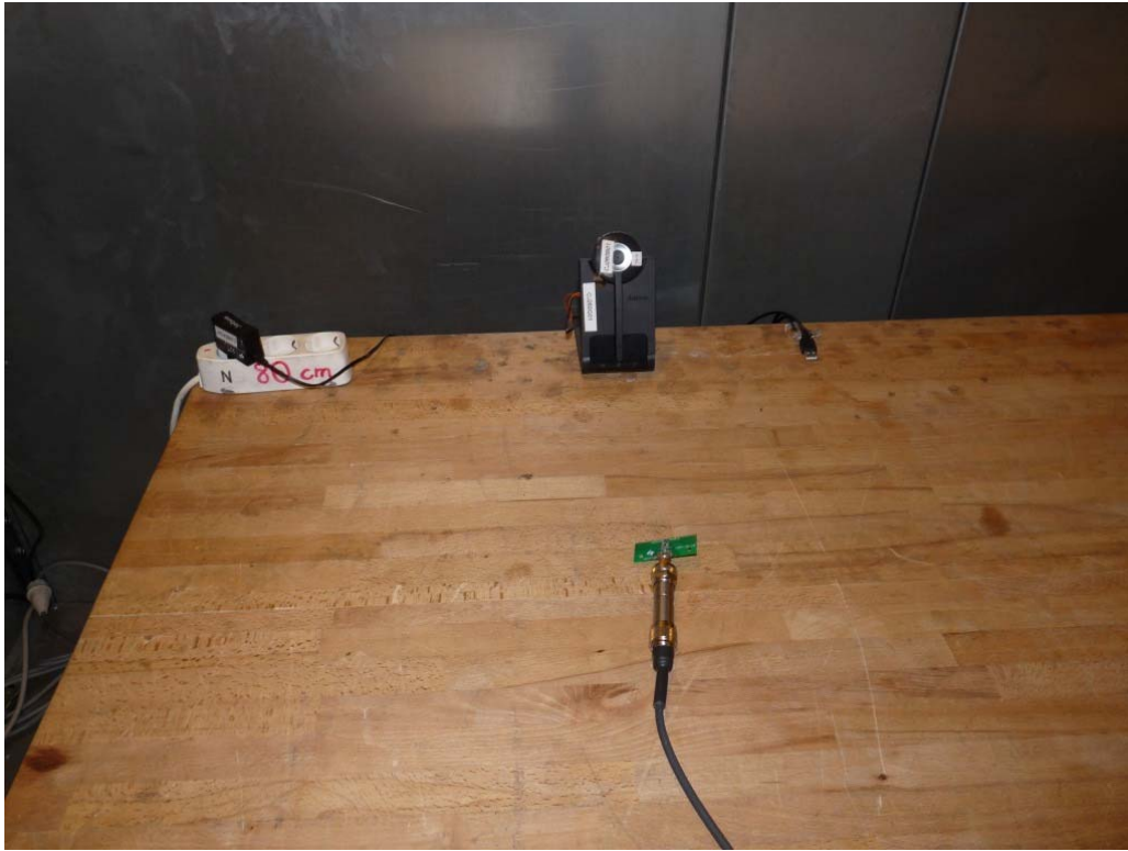
Photo 1: Test setup for conducted measurements (AC Port (power line), EUT supplied by AC/DC adapter, intentional / unintentional radiator §15)
