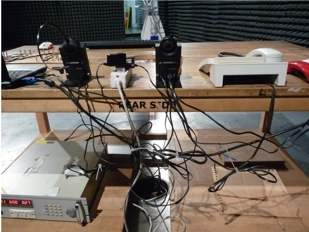
Photo 4: Test setup for radiated measurements (AC Port (power line and computer peripheral setup), EUT supplied by AC/DC adapter. Data traffic on USB-Cable by streaming music, unintentional radiator §15)
