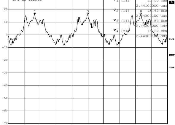
Center 2.442 GHz 300 kHz/ Span 3 MHz
