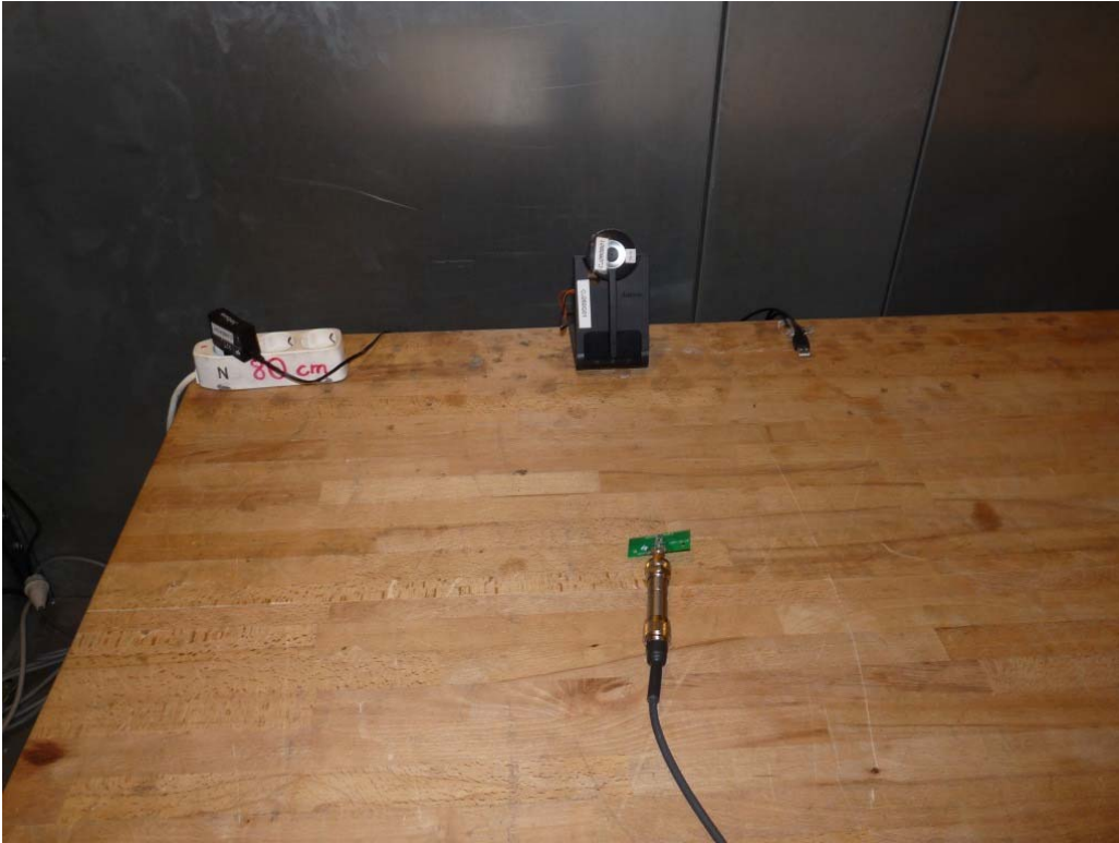
Photo 5: Test setup for conducted measurements (AC Port (power line), EUT supplied by AC/DC adapter, intentional / unintentional radiator §15)
