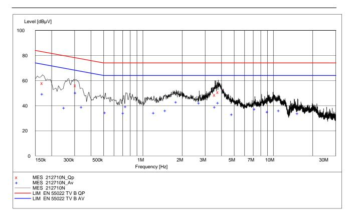
EUT On-Hook, Charging, Base powered from USB
