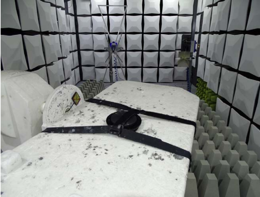
Photo 9: Test setup for radiated measurements in the range 1 – 26 GHz, used for intentional radiator measurements.
