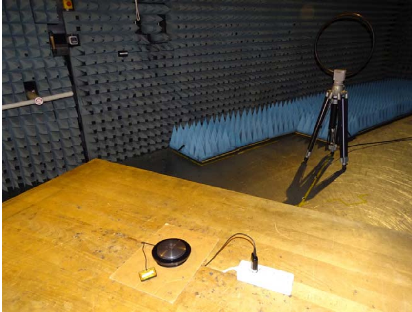
Photo 7: Test setup for radiated measurements in the range 9 KHz – 30 MHz, used for intentional radiator measurements.
