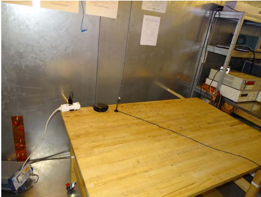
Photo 1: Test setup for conducted measurements on AC port, standalone setup, EUT supplied by AC/DC adapter, USB connected, used for intentional and unintentional radiator measurements.
