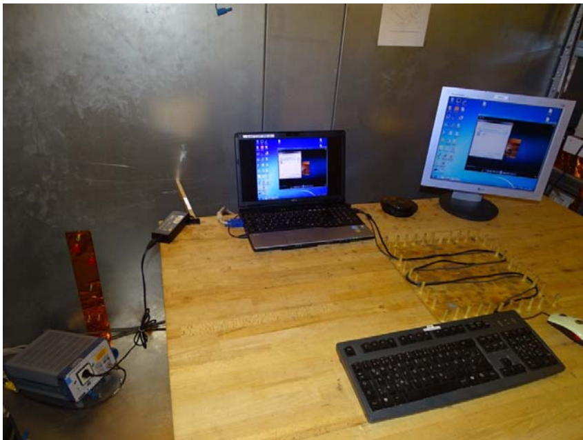
Photo 1: Test setup for conducted measurements on AC port, computer peripheral setup, EUT supplied by computer, USB connected, used for unintentional radiator measurements.
