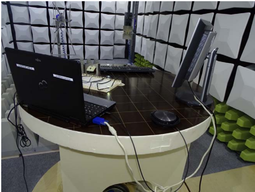
Photo 8: Test setup for radiated measurements in the range 1-13 GHz, used for unintentional radiator measurements.
