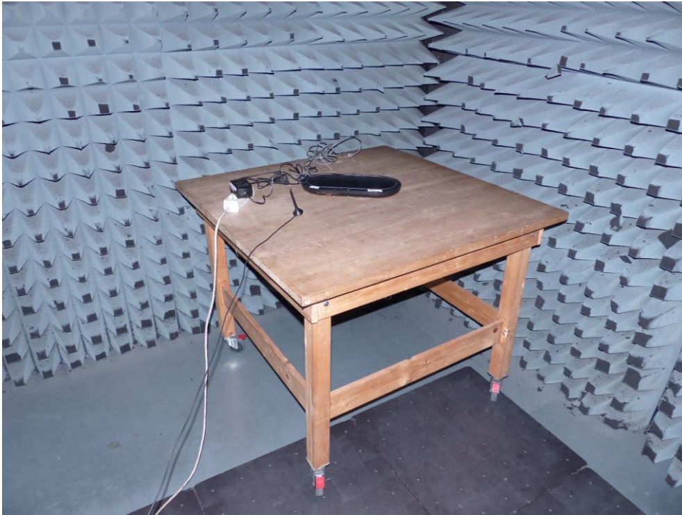
Photo 7: Test setup for radiated measurements below 30 MHz, used for intentional radiator measurements.
