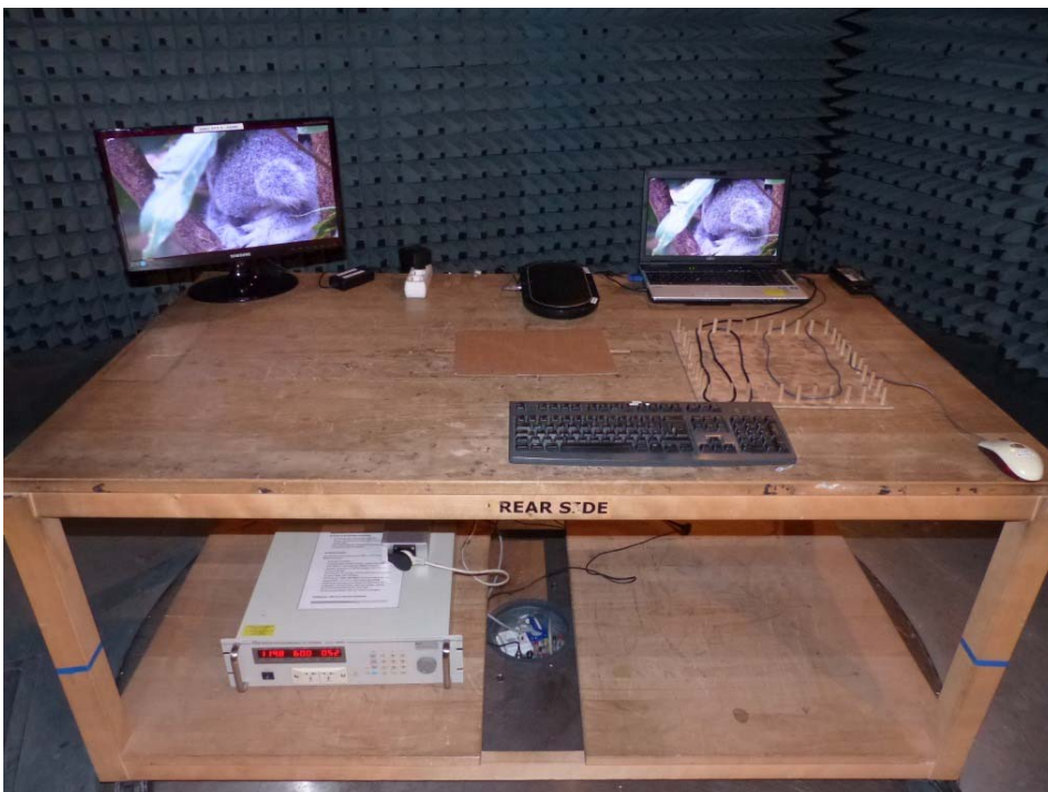
Photo 4: Test setup for radiated measurements in the range 30 – 1000 MHz, EUT supplied by AC/DC adapter, computer peripheral setup, used for unintentional radiator measurements.
