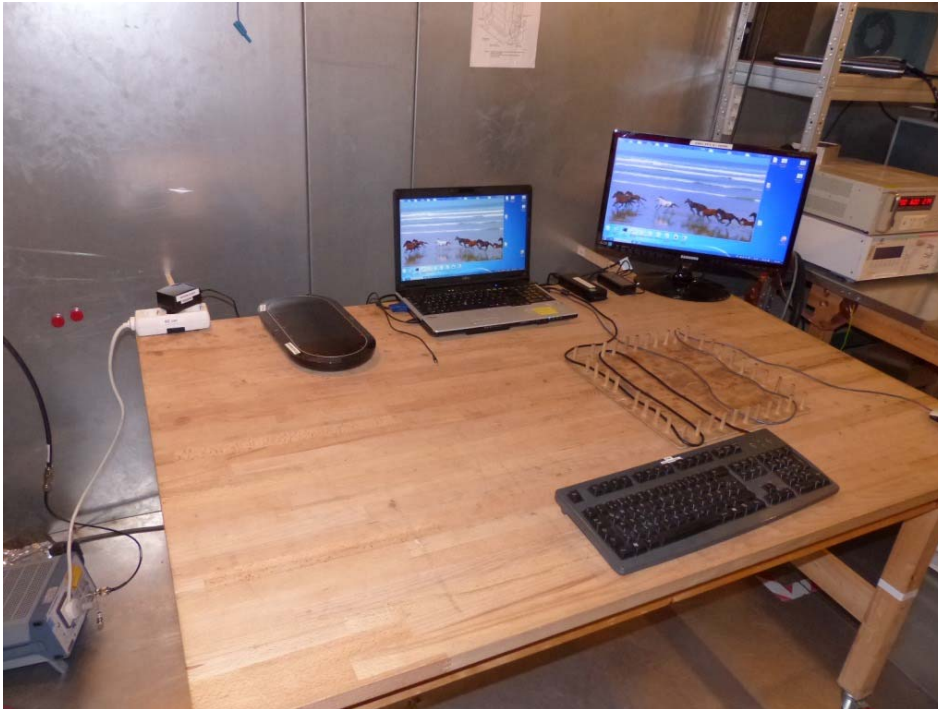
Photo 1: Test setup for conducted measurements on AC port, computer peripheral setup, EUT supplied by AC/DC adapter, USB connected, used for intentional and unintentional radiator measurements.
