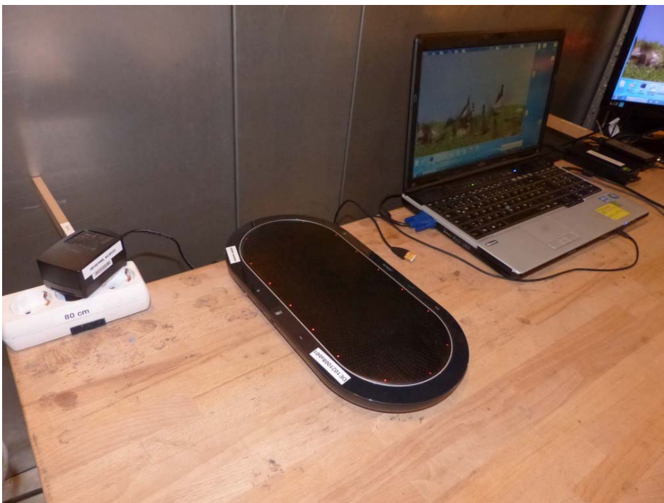
Photo 2: Test setup for conducted measurements on AC port, computer peripheral setup, EUT supplied by AC/DC adapter, Clinch connected, used for unintentional radiator measurements.
