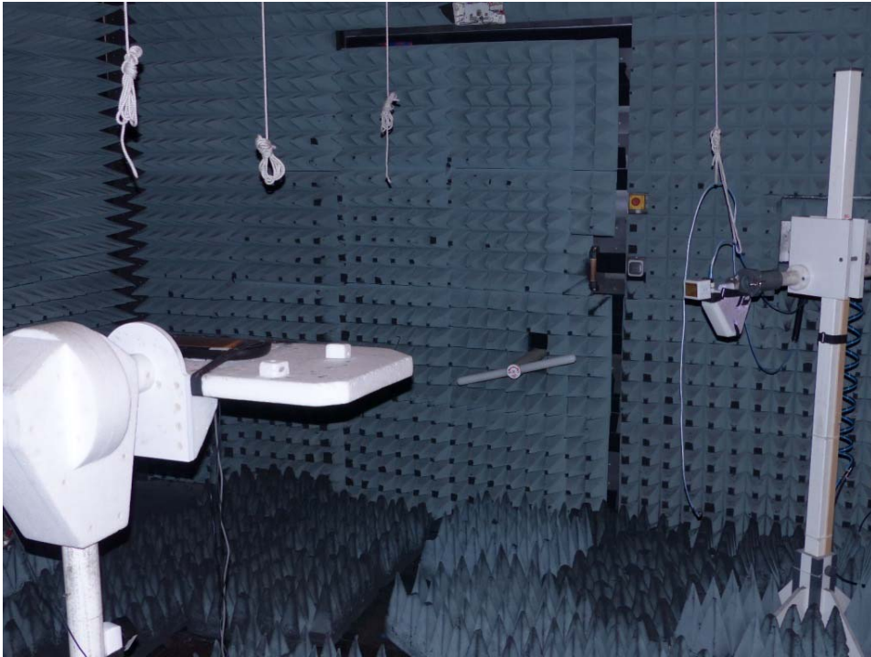
Photo 9: Test setup for radiated measurements in the range 18 – 25 GHz, fully-anechoic chamber, used for intentional radiator measurements.
