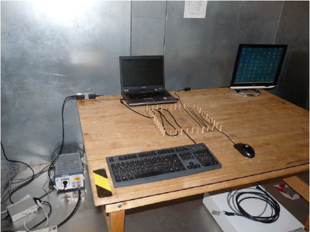
Photo 5: Test setup for conducted measurements (AC Port (power line)), unintentional transmission, EUT + computer peripheral setup
