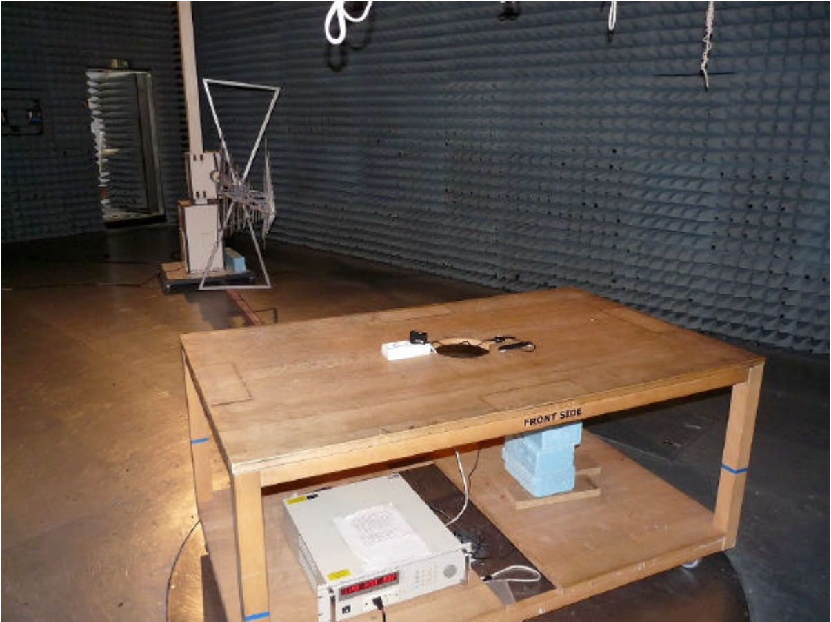
Photo 6: Test setup for radiated measurements (Enclosure, 30 MHz to 1 GHz), unintentional transmission, EUT + AC/DC adapter
