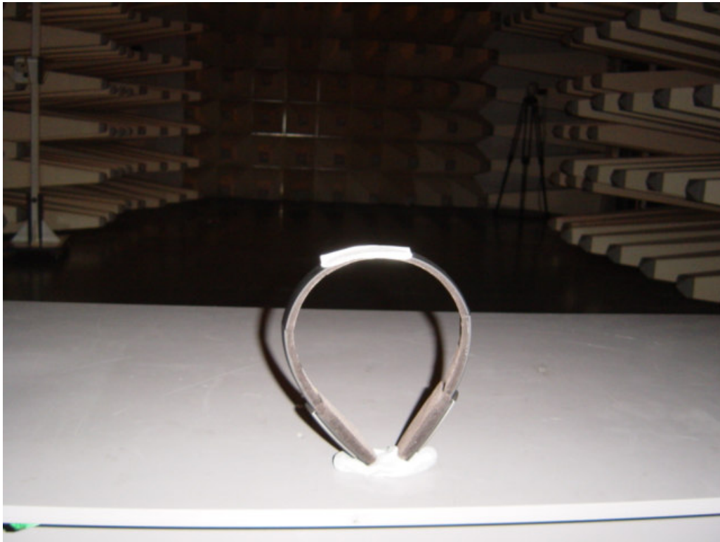
Set-up for Radiation Emission (Transceiver)
