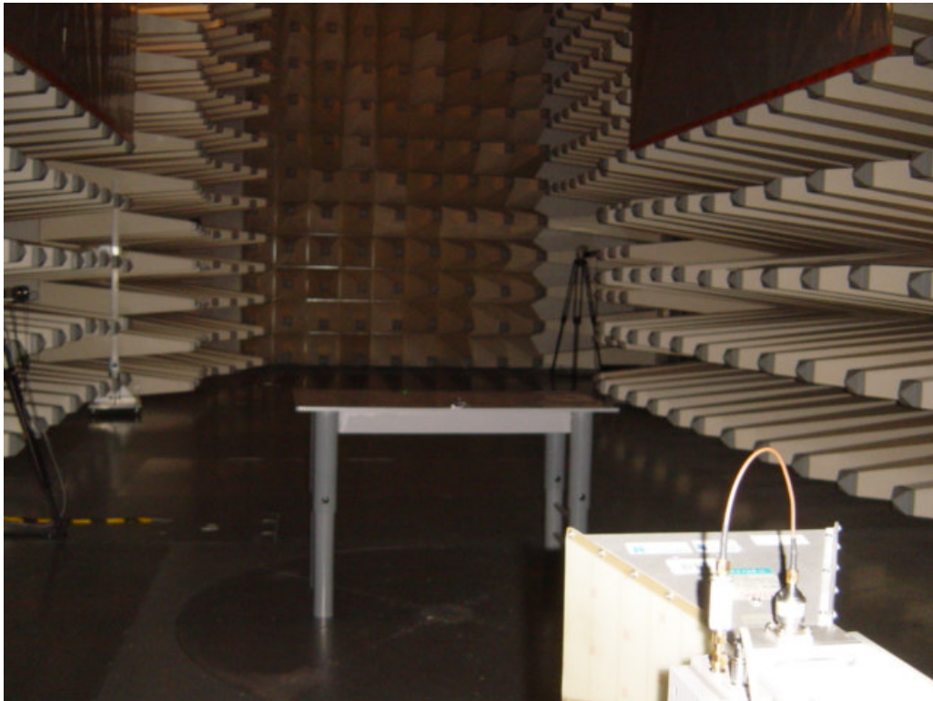
Set-up for Radiation Emission (Transceiver)
