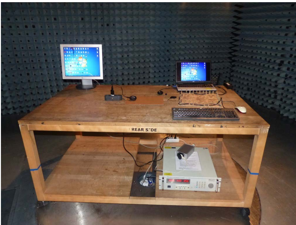
Photo 4: Test setup for radiated measurements (Semi Anechoic Chamber, EUT supplied by computer, 30 – 1000 MHz, intentional & unintentional radiator §15)
