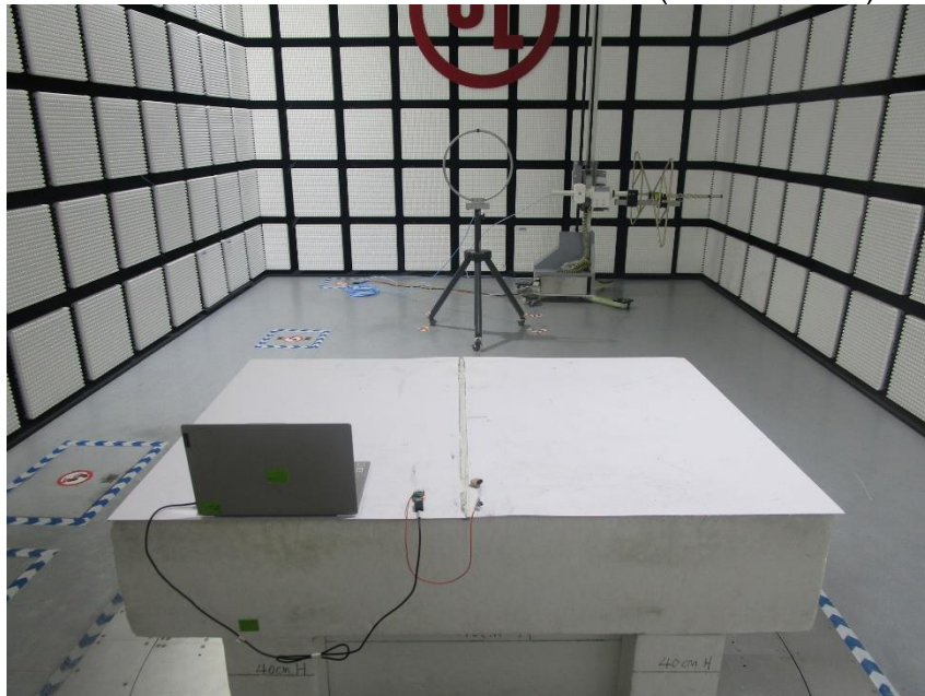
RADIATED RF MEASUREMENT SETUP (Below 30MHz)
