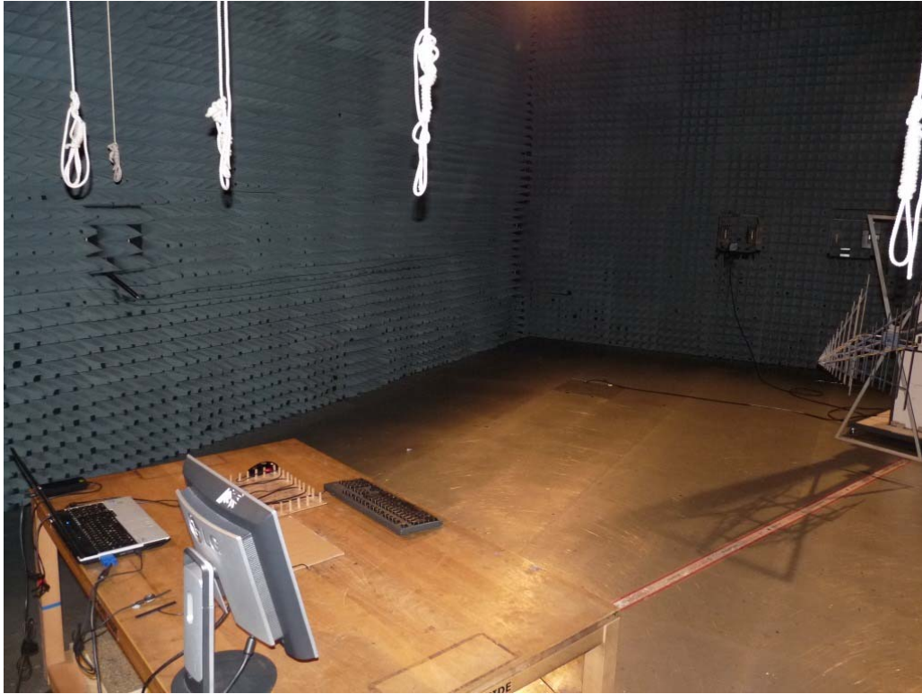
Photo 2: Test setup for radiated measurements (computer peripheral setup, EUT supplied by USB-cable from computer, unintentional radiator §15)
