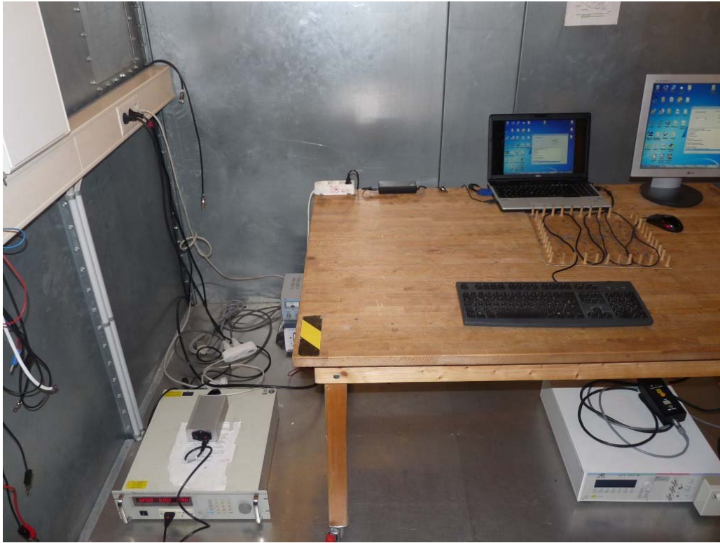
Photo 1: Test setup for conducted measurements (computer peripheral setup, EUT supplied by USB-cable from computer, unintentional radiator §15)
