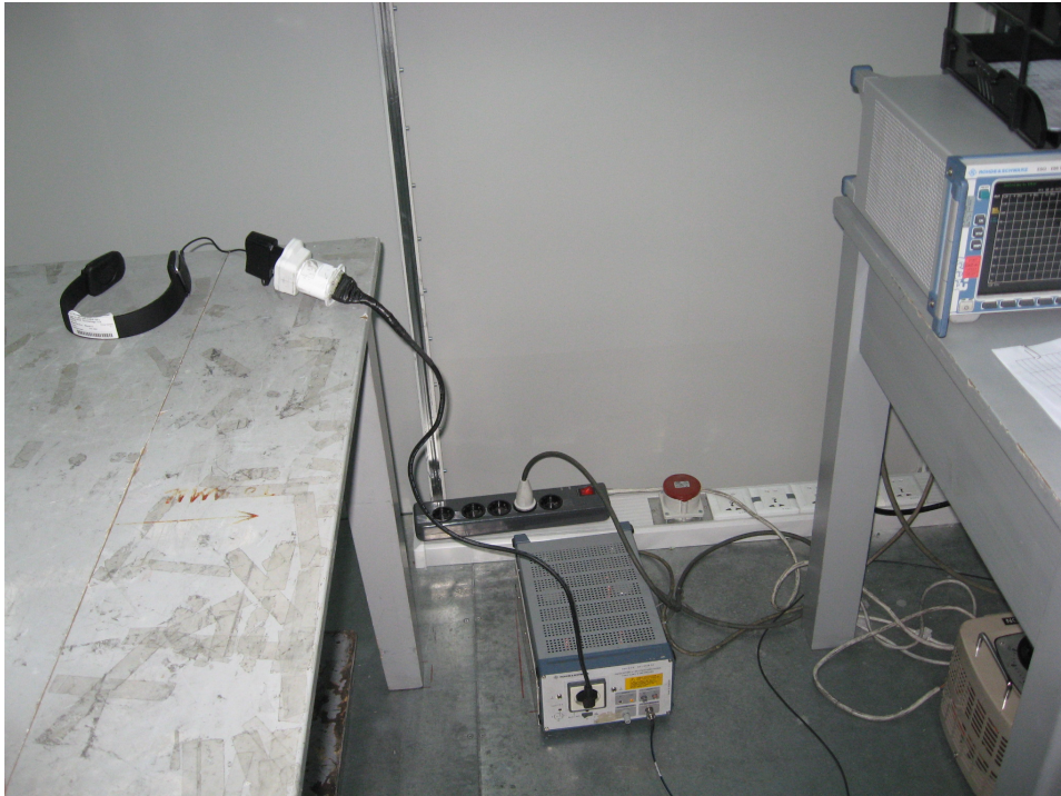
Test Setup for Conducted Disturbance Measurement
