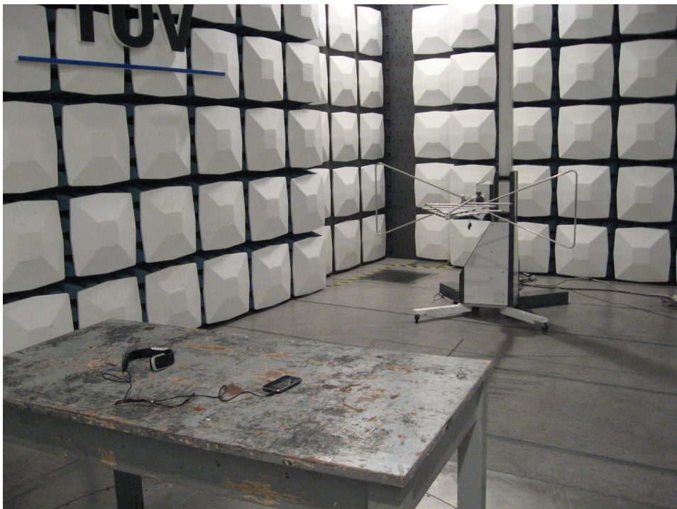
Test Setup for Radiated Disturbance Measurement
