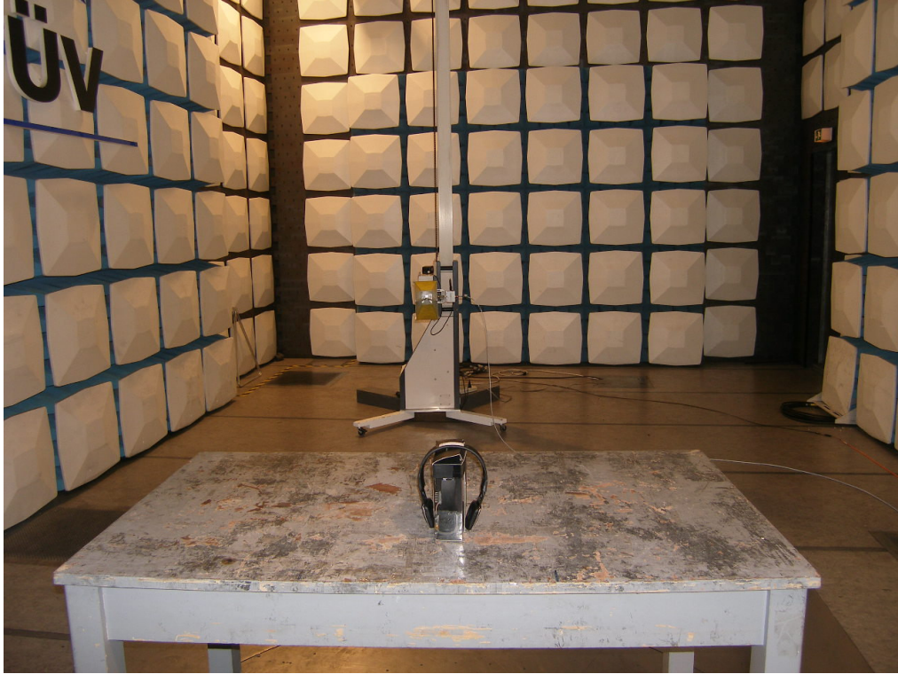
Setup for Radiated Emission
