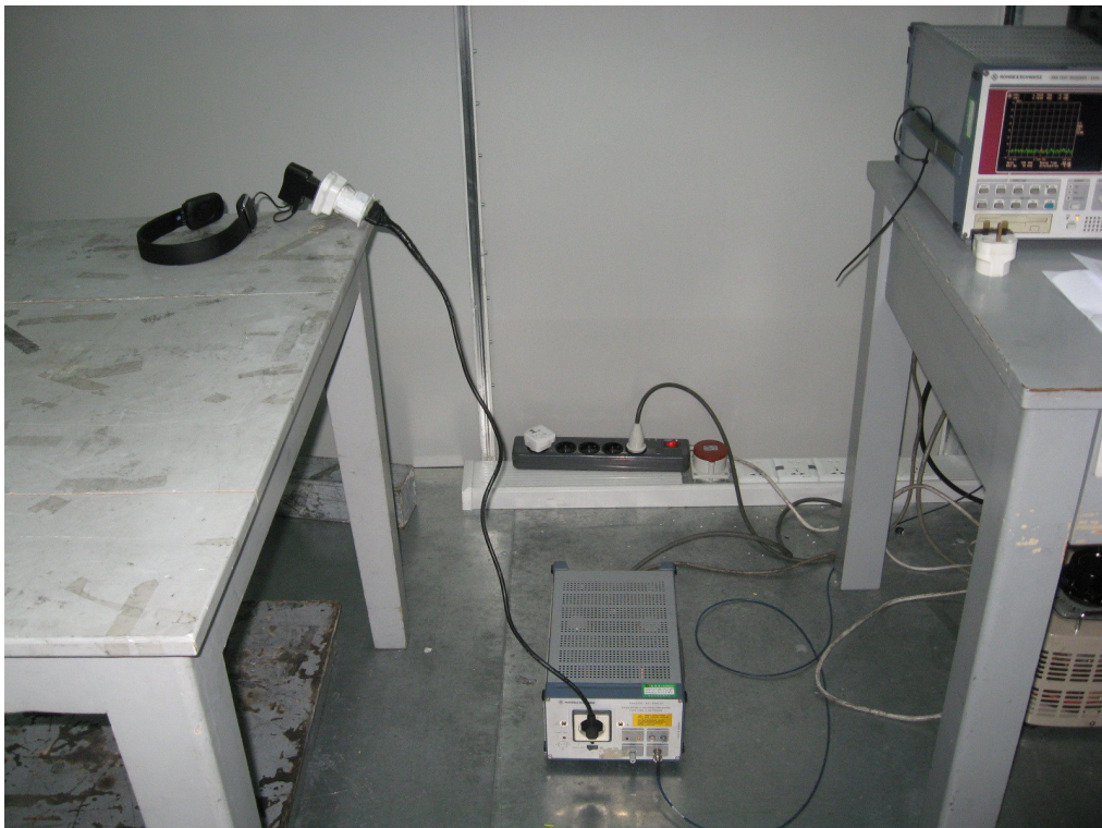
Setup for Conducted emission - AC mains input/output port
