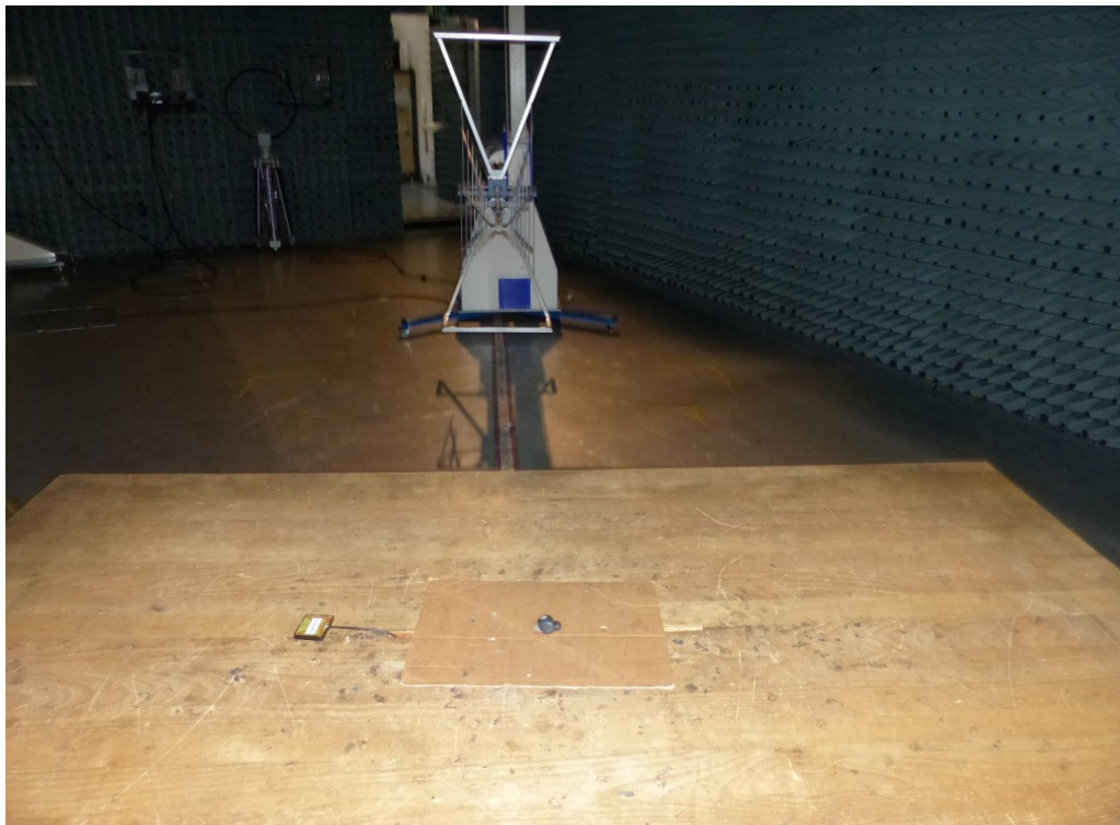
Photo 4: Test setup for radiated measurements.
