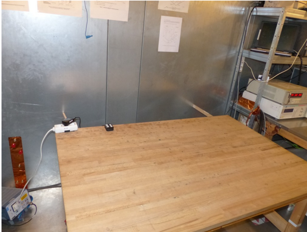
Photo 5: Test setup for radiated measurements
