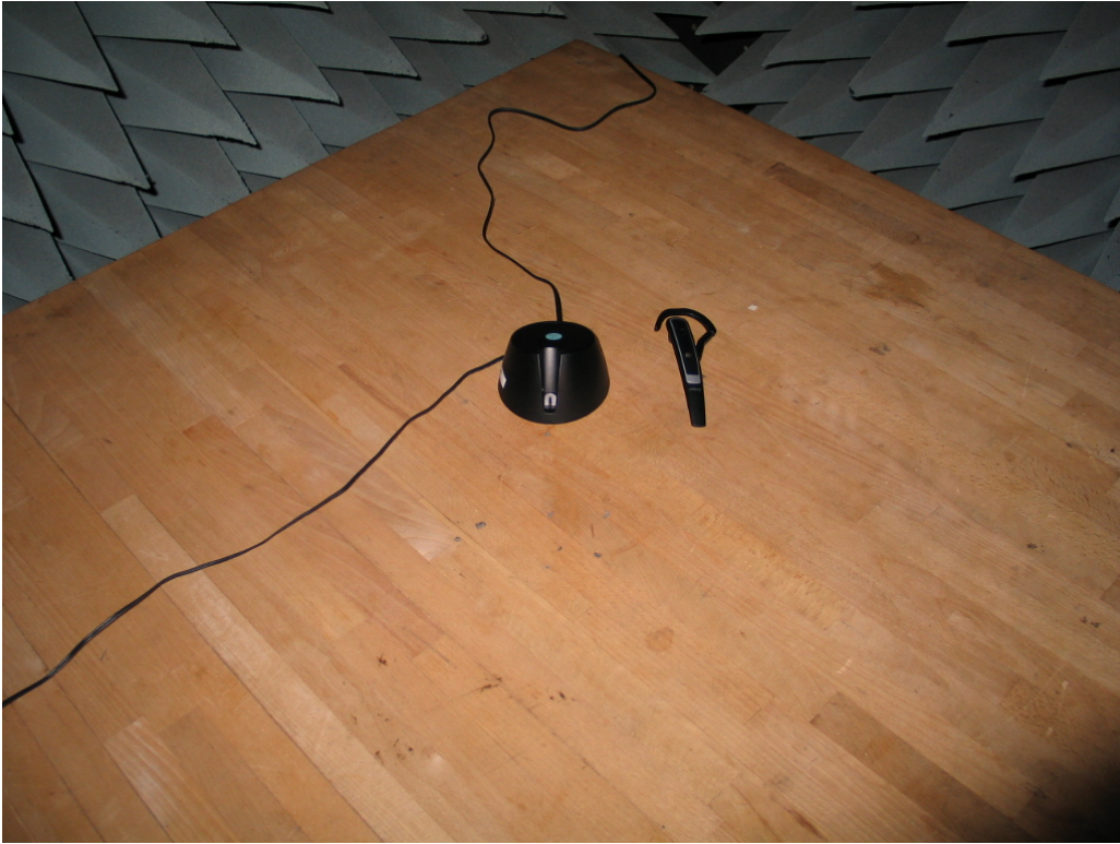
Photo 1: Test setup for radiated measurements (Enclosure, Setup_c01, below 30 MHz)
