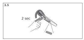
3.5 Turn the headset on by pressing the Answer/End button for 1 sec. (the visual indicator will flash blue four times and headset will beep three times), or by placing headset in charge cradle. Turn the headset off by pressing the Answer/End button for 2 sec. (visual indicator will flash blue four times and headset will beep three times).
