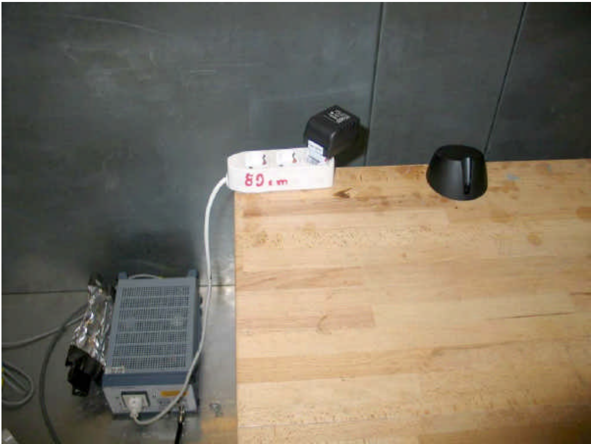
Photo 4: Test setup for conducted measurements (AC Mains)
