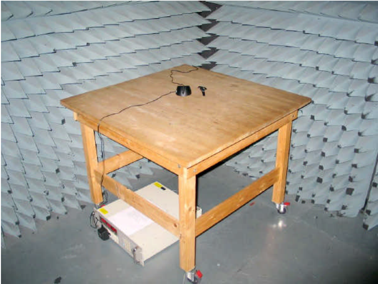
Photo 3: Test setup for radiated measurements (below 30 MHz)
