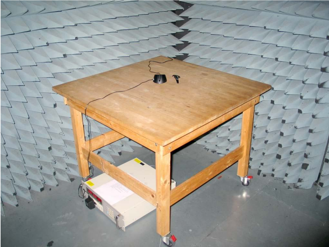
Photo 3: Test setup for radiated measurements (below 30 MHz)
