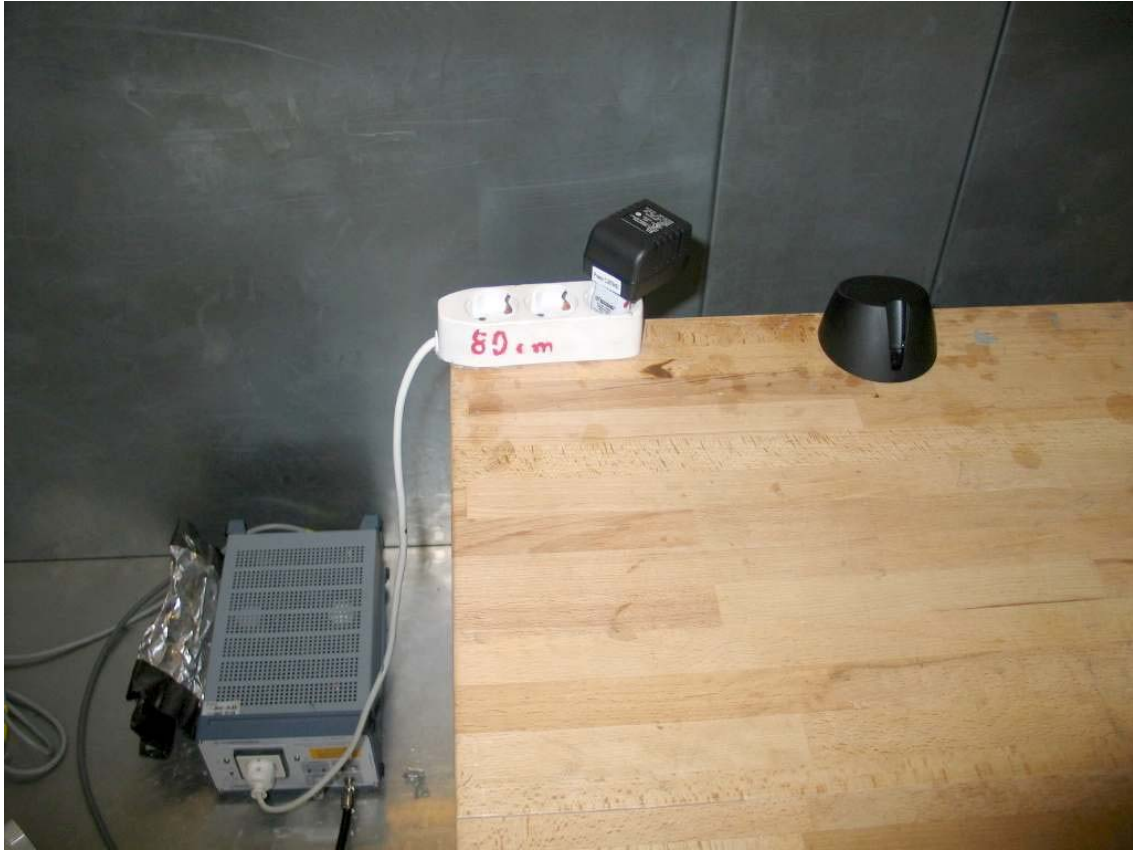
Photo 4: Test setup for conducted measurements (AC Mains)
