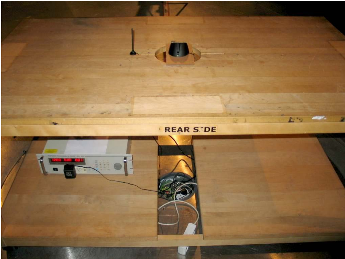
Photo 2: Test setup for radiated measurements (between 30 MHz and 1 GHz)
