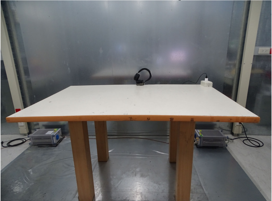
Front View of Conducted Test –Charge Mode
