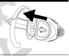
2 Gently lift and pull the top of the earhook up and off the upper hinge pin. Then pull it away to remove it.
