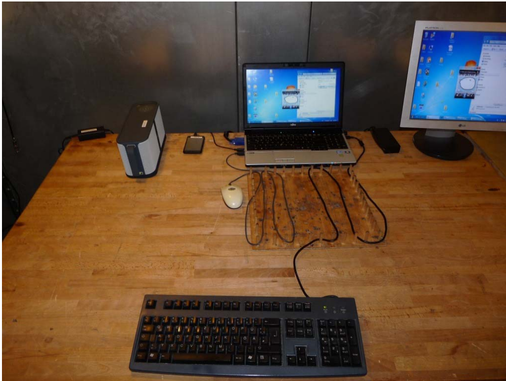
Photo 1: Test setup for conducted measurements (computer peripheral setup, EUT supplied by AC/DC Adapter. USB-cable from computer used for streaming music, USB cable to mobile phone for charging) unintentional radiator §15)
