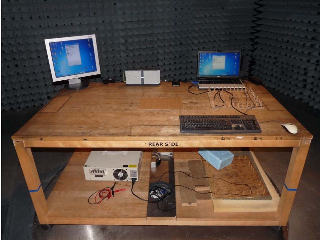
Photo 2: Test setup for radiated measurements (computer peripheral setup, EUT supplied by AC/DC Adapter. USB-cable from computer used for streaming music, USB cable to mobile phone for charging), unintentional radiator §15)
